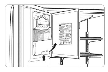
To reinstall the in-door ice bin, slightly slant the bin during replacement to avoid contact with the icemaker.
